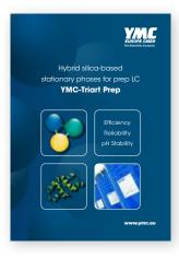
Hybrid silica phase, stable between pH 2.0–10.0 Available with C18 and C8 bonding.
