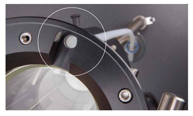
Bubble-free piston insertion due to the smart drain function – smooth packing process, guaranteeing a well packed column for great chromatographic performance!
